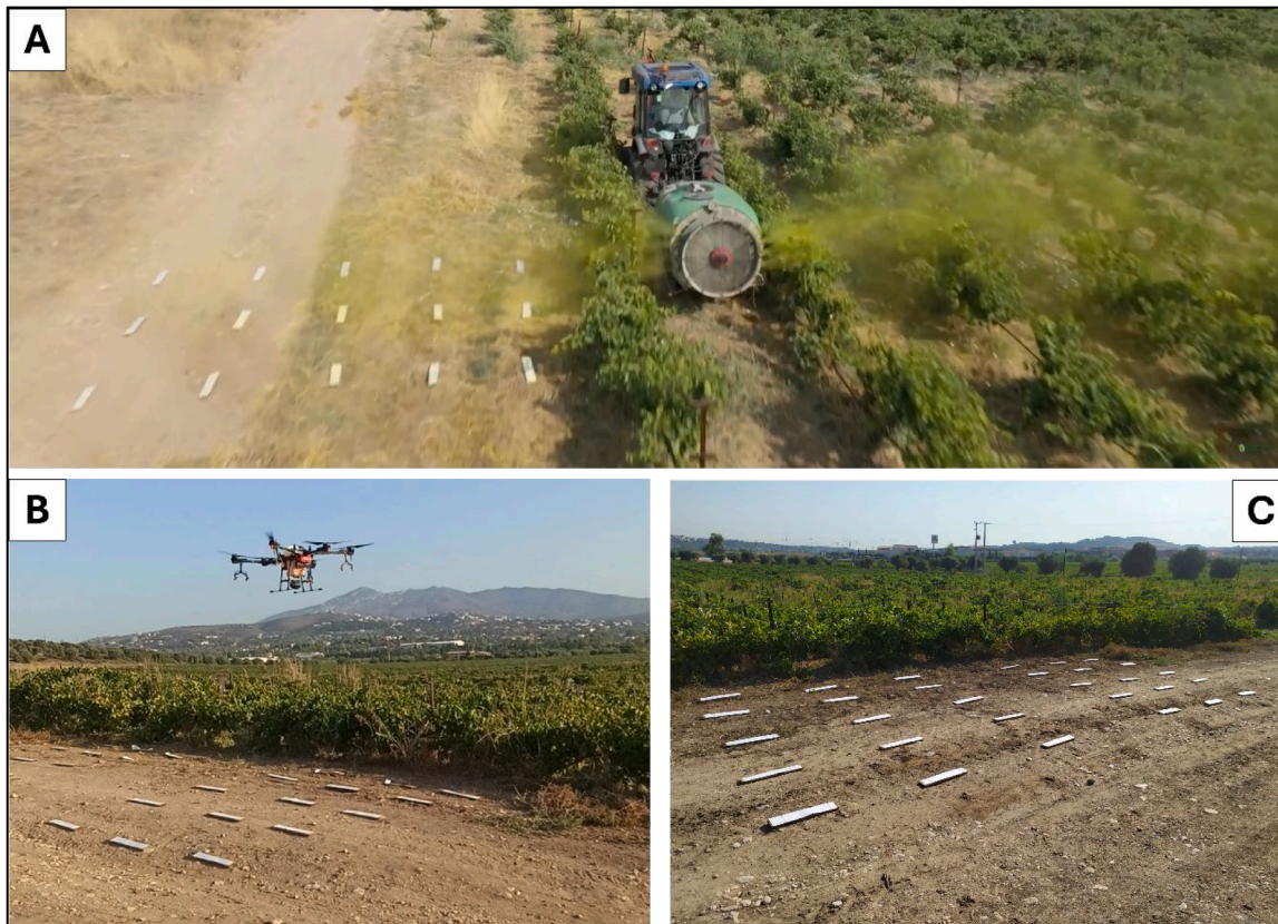
Fig. 2. (A) The conventional air-assisted sprayer used in the trials, (B) the spraying UAV used in the trials, and (C) an overview of the first 5 m of the sampled area.
